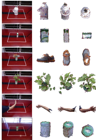
Fig. 7. Reconstruction results. Each row shows an reconstruction example with color images and three views of reconstructed point clouds.
